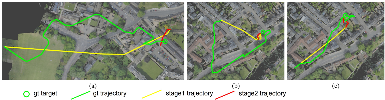
Figure 4: Visualization results for the two-stage navigation. Initial predictions in the coarse-grained stage may exhibit target drift or premature stopping. The fine-grained refinement stage corrects these deviations and steers the agent toward the ground-truth target. Three representative cases are visualized to illustrate this behavior.
